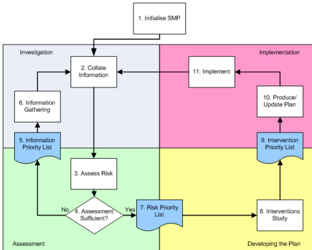
Figure 1 SRM Procedure
