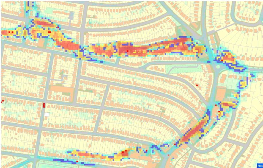
This example is from the FRM tool, which represents the obstruction to the flow caused by buildings. There are therefore islands within the flow paths where there is no flooding as they are under buildings.
