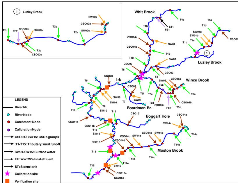
Figure 3. Schematic representation of the MIKE BASIN model of the River Irk.
