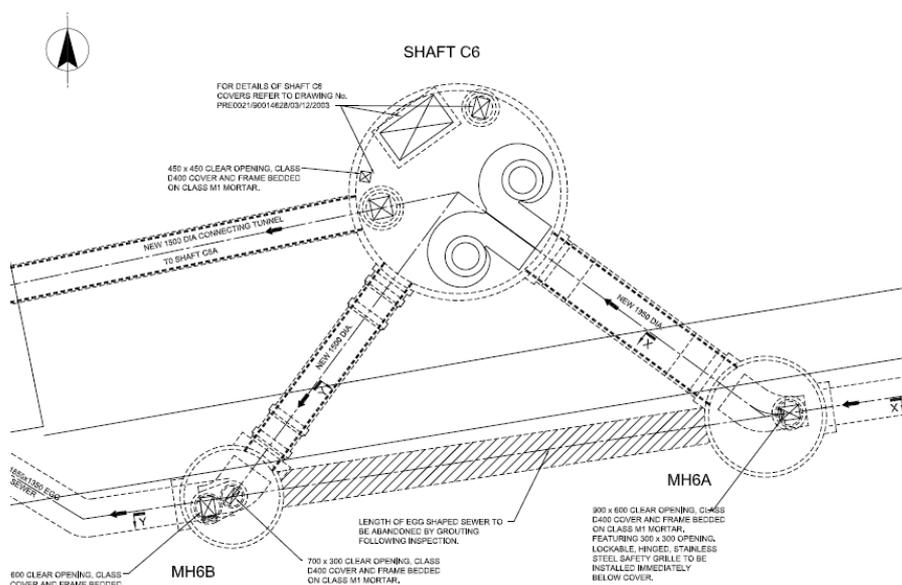
Diagram showing the details of a connection at one of the drop shafts
