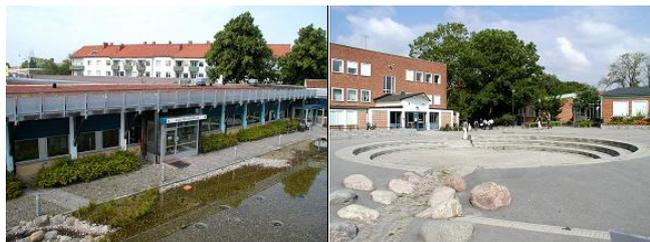
*Figure 1 Temporary detention pond in urban environment (right). and green roof on a building (left)*
