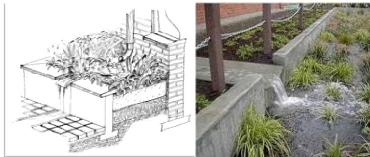
Figure 2 (left) An example of an infiltration planter collecting water directly from the roof (courtesy Timber Press, Dunnett & Clayden 2007). Figure 3 Portland Oregon: Mt. Tabor Middle School Rain Garden (Photo Credit: Mt. Tabor Middle School)
