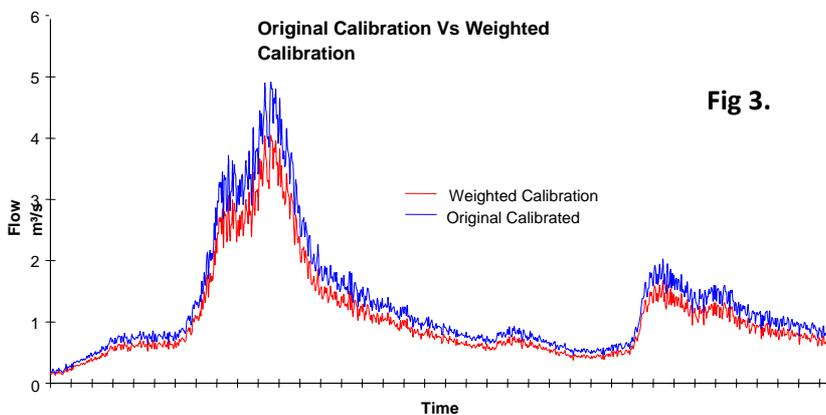
This highlights the significant potential for inaccuracies (as large as the verification criteria bands!) in the observed data in large sewers due to this aspect of the flow calculation and calibration when using single point velocity monitors.
