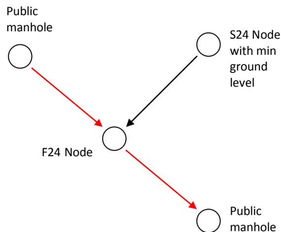
Figure 3.0 Illustration of simplified formerly private drainage network (lateral connection)
