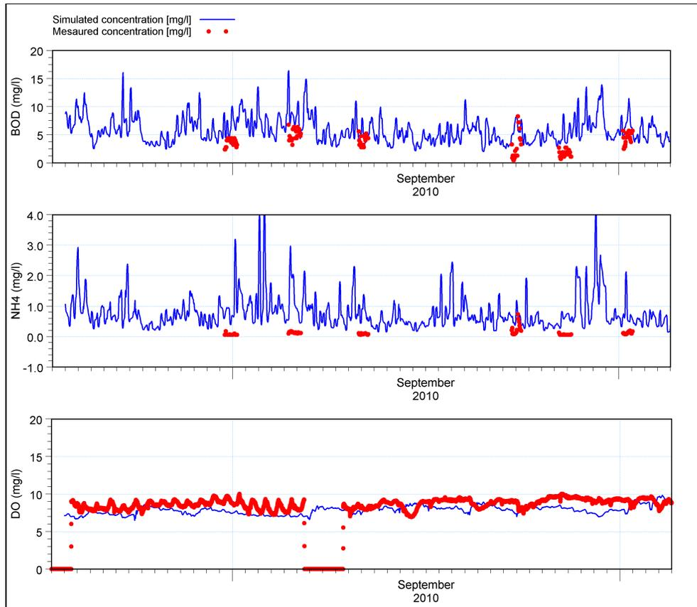
**Figure 7. Verification results at Wanes Blades on the River Douglas for the period August-September 2010.**
