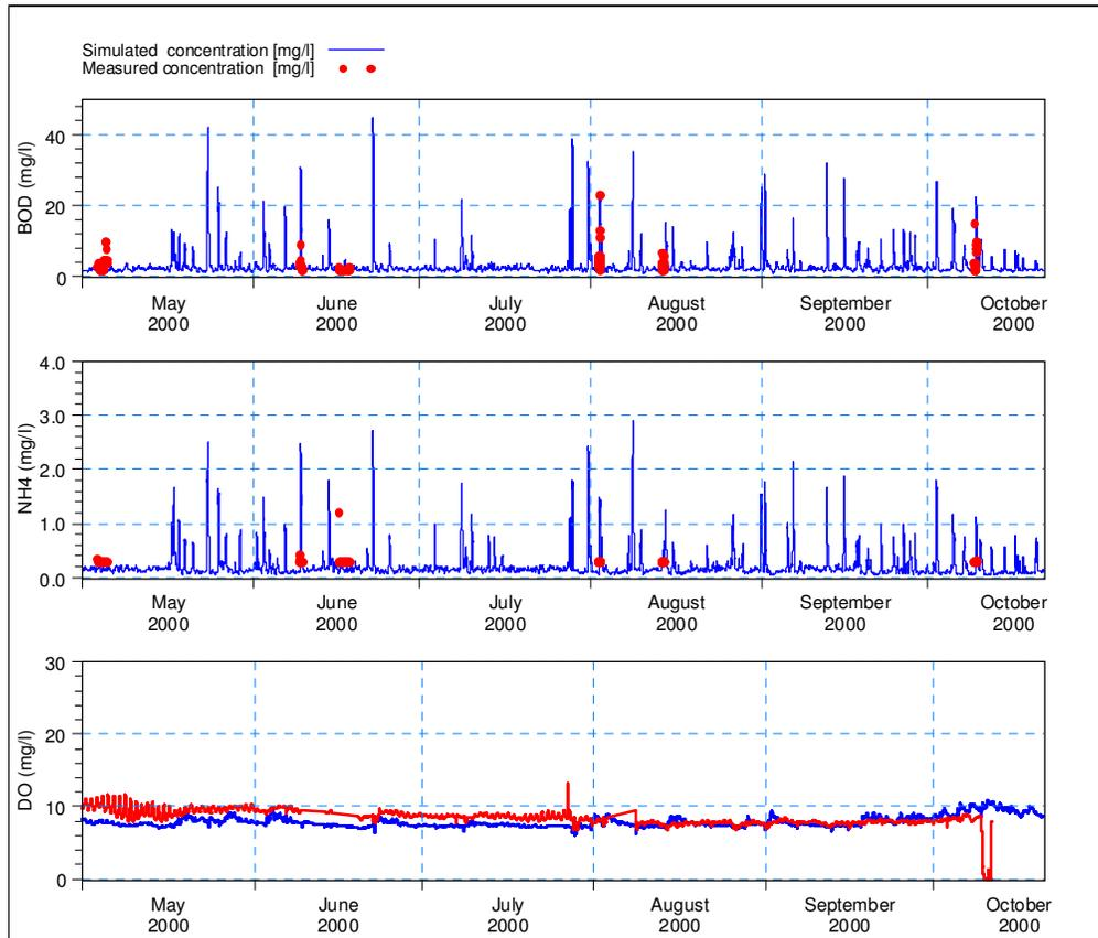
**Figure 6. Verification results at Leyland Mill Bridge Lane on the River Douglas for the period May-October 2000.**
