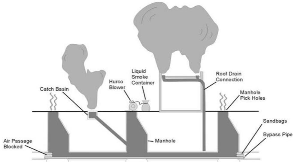
**Figure 4 – Smoke Testing Site Process**
