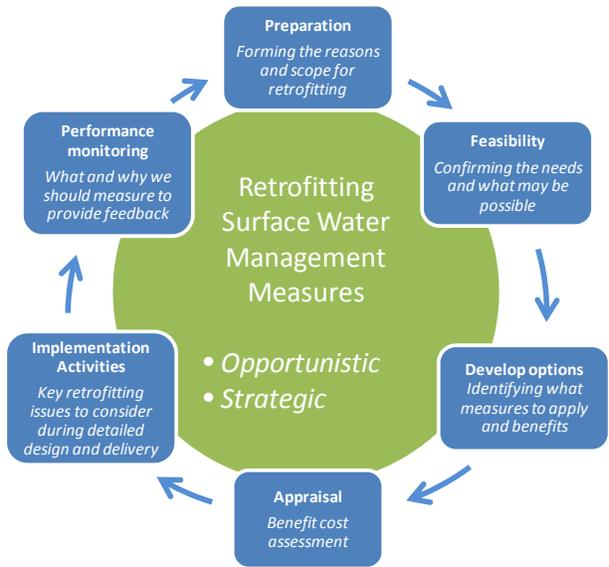
Figure 1 The retrofitting surface water management framework
