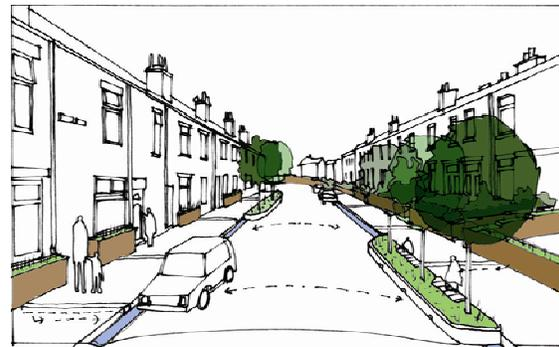
Figure 3 (courtesy of CIRIA) Managing water on the surface with shallow above ground channels, planters & bio-retention areas
