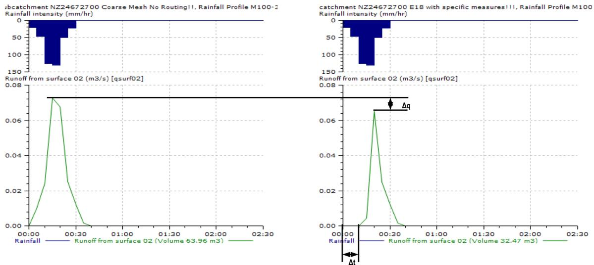
Figure 3 Demonstration of the effects of the SuDS on the runoff hydrographs
