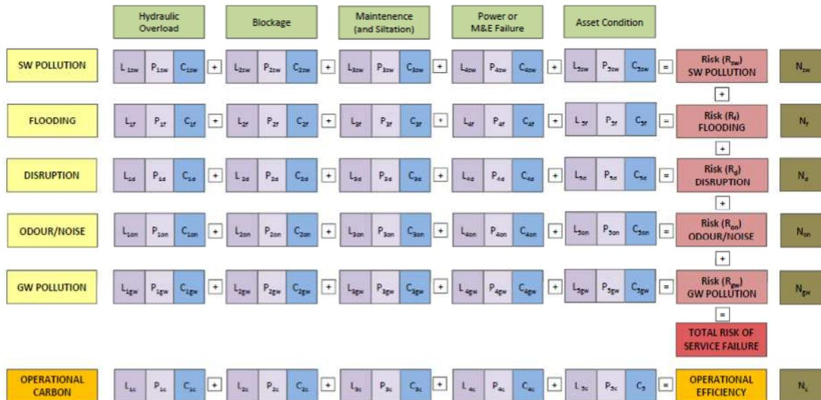
Figure 3 – SRM Risk Methodology Matrix – Wastewater Assets
