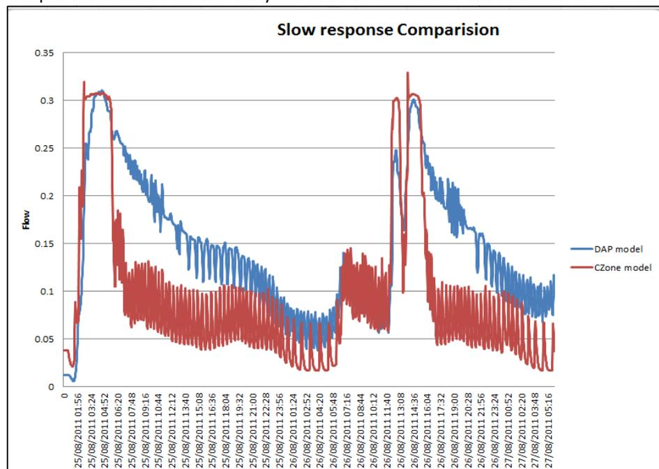
Figure 3: Observed WFD response (red) vs. predicted DAP model response (blue). WFD and DAP model are both considered verified to their respective flow surveys
