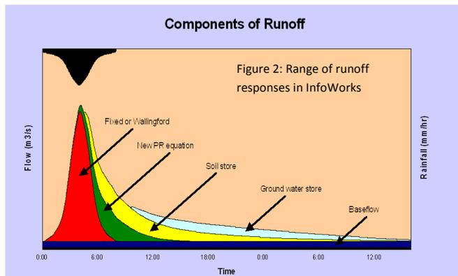
A Comparison of the various runoff modules available in InfoWorks CS indicated that the very slow response observed on the foul system may potentially be due to contributions from the Ground Store. By altering the properties of the two different Soil Store only profiles to replicate the highly attenuated observed flows the runoff contributions from the ground store, which had not been utilised at this stage, were being replicated through the application of dummy area.
