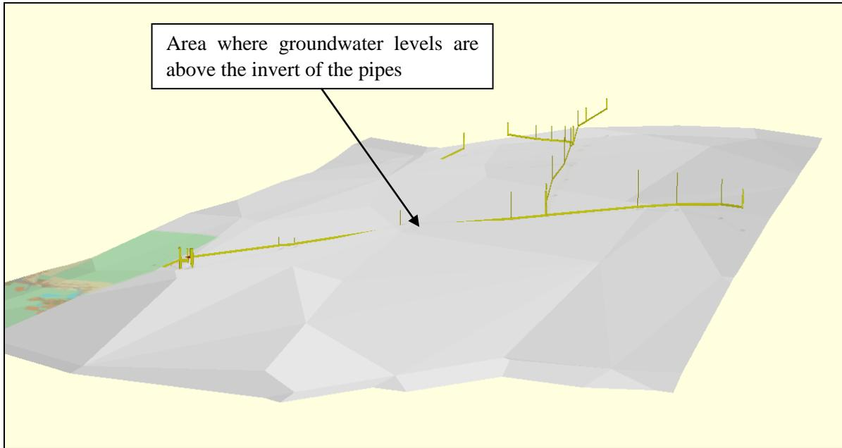
**Figure 4.3 – Comparison of maximum groundwater levels to pipe inverts**
