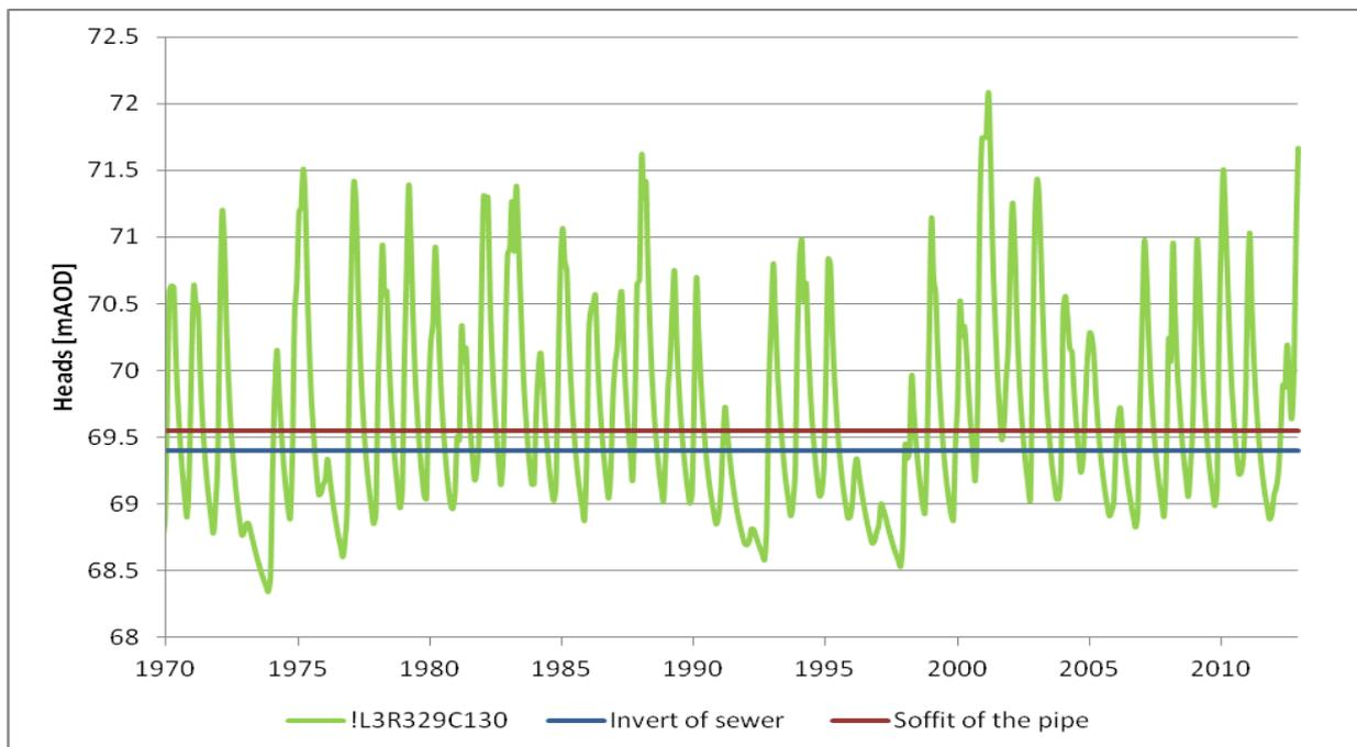
**Figure 4.4: Groundwater level against pipe invert level over the full range of the model**
