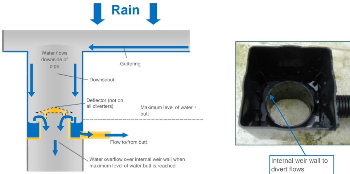
**Figure 1 – Basic principles of a rain diverter.**
