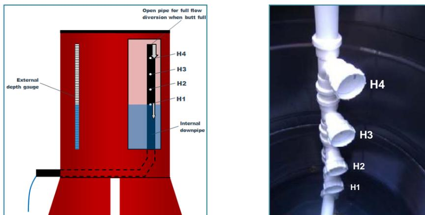
Figure 6 & 7 – Internal discharge arrangements.
