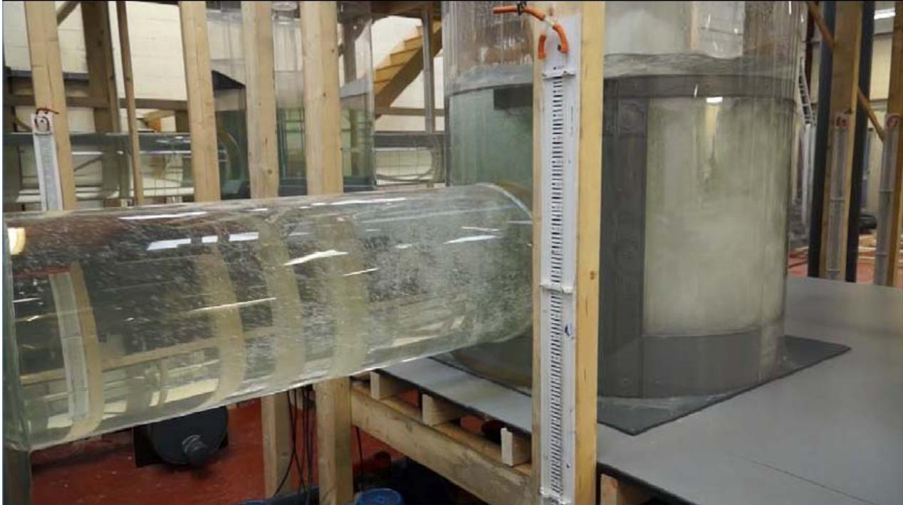
Figure 8 – Testing of the tangential intake vortex drop (3), de-aeration chamber for the 1 in 30 year return period flow with tunnel full. Note the bubble track rapidly directs air to the soffit
