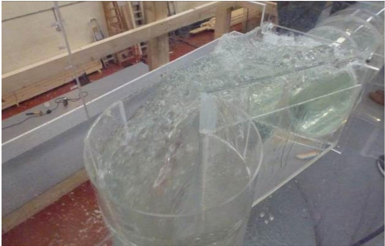
Figure 6 – Testing of the tangential intake vortex drop (1), flow entering the vortex drop under critical conditions
