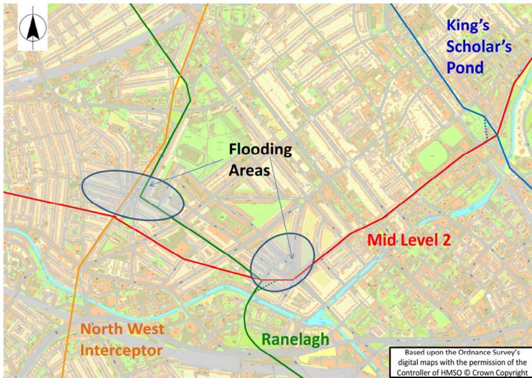
Figure 1 – Location of flooding in the Maida Vale area and trunk sewers.
