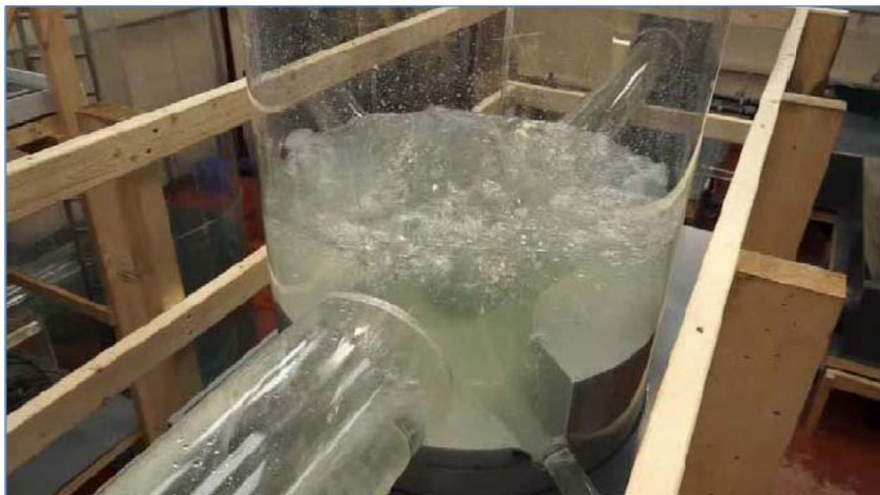
Figure 7 – Testing of the tangential intake vortex drop (2), control point for the flow upstream and substantial head losses
