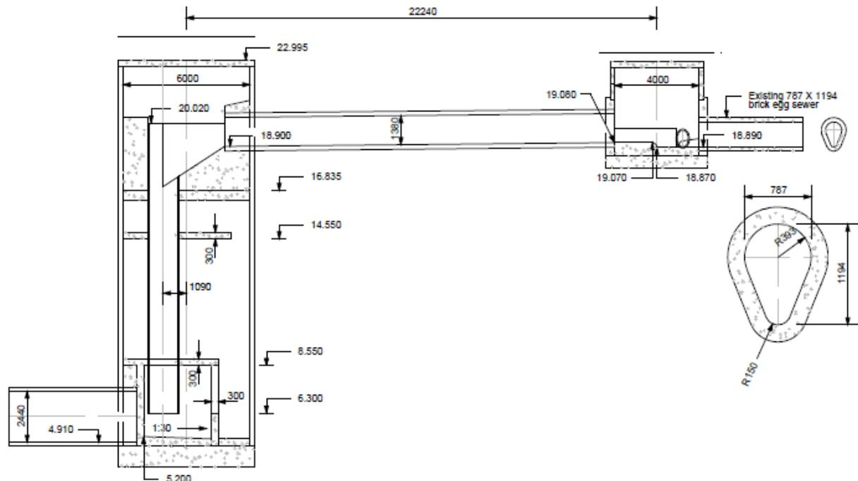
Figure 5 – Drawing showing the section of the drop shaft and upstream manhole
