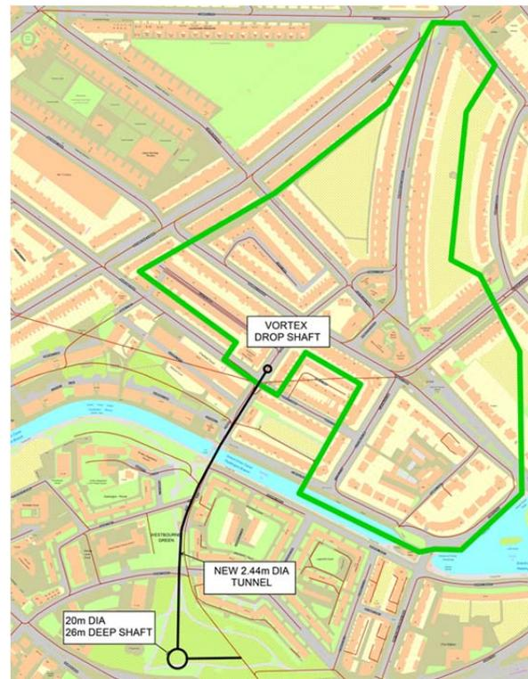
Figure 2 – Overall scheme to solve the Maida Vale flooding
