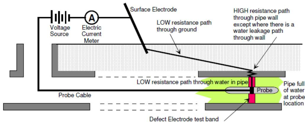
**Figure 1: Simplified Circuit Diagram of Electronic Survey**
