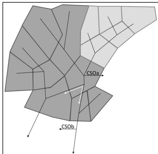
Figure 2 – Catchment 2, part of a complex sewer catchment with multiple CSOs, a bifurcation and combined and separate systems.
