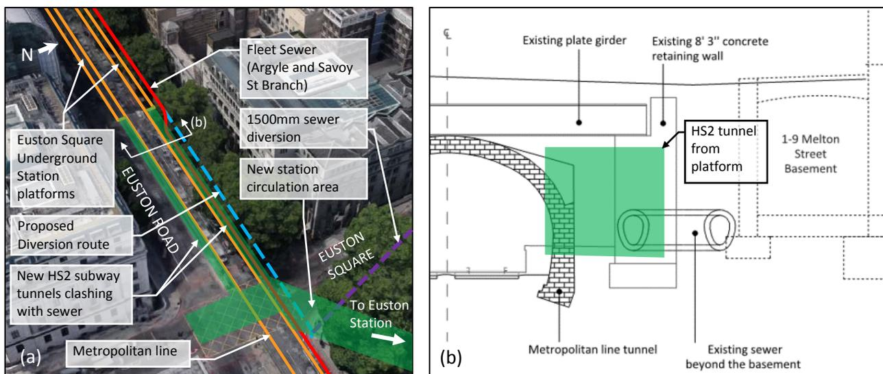
Figure 4 - (a) The Fleet Sewer (Argyle and Savoy Street branch) in Euston Road showing the Metropolitan Line and the sewer diversion route (Google Maps imagery) (b) Cross section (looking west along Euston Road) of the sewer, basement and Euston Square Underground Station (courtesy of HS2)
