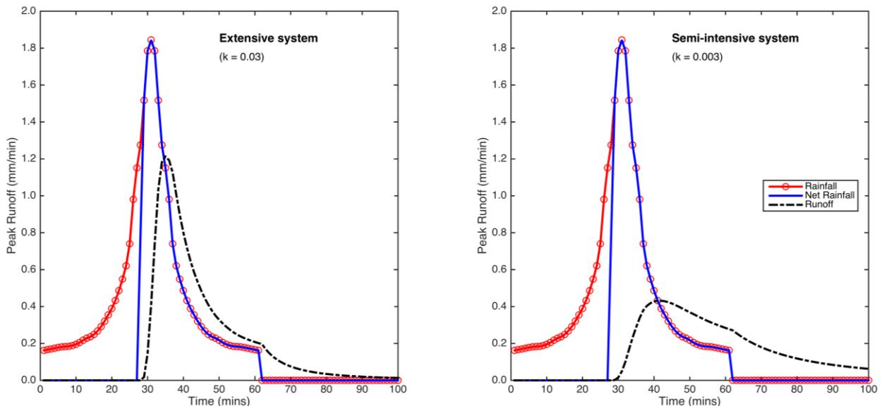
**Figure 3 Detention for design storms with 30 mm rainfall and 10 mm retention capacity**
