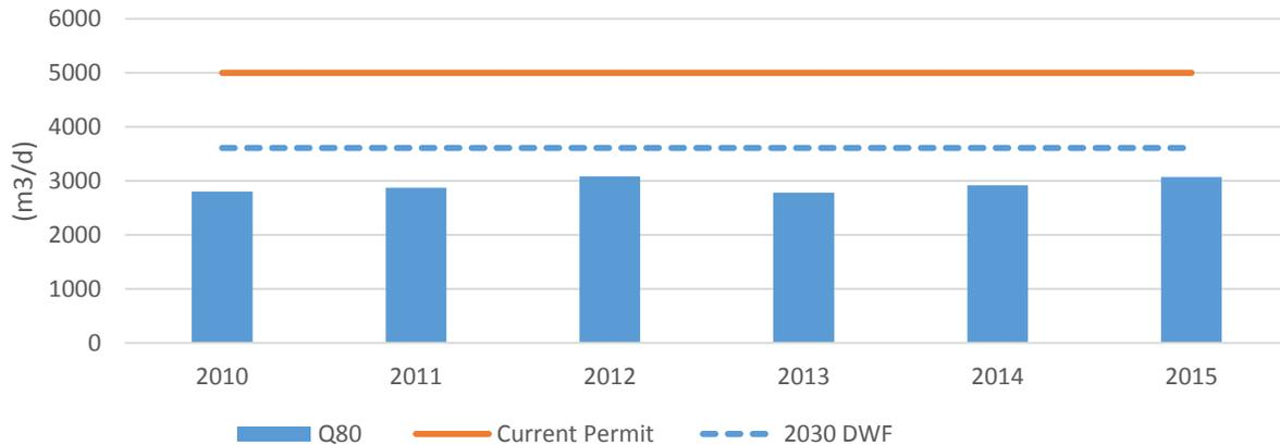
**Figure 2 – An example output of a simplified analytic to continuously calculate Q80 flow from a STW**
