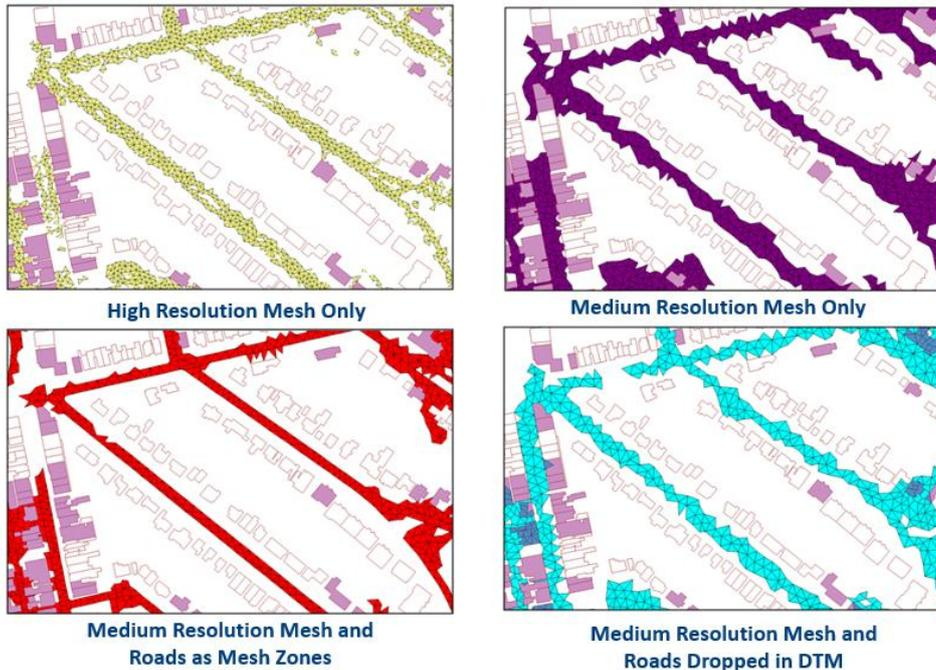
Figure 3: shows a comparison of the modelled overland flows and the impact on predicted risk when different methods are used to represent roads.
