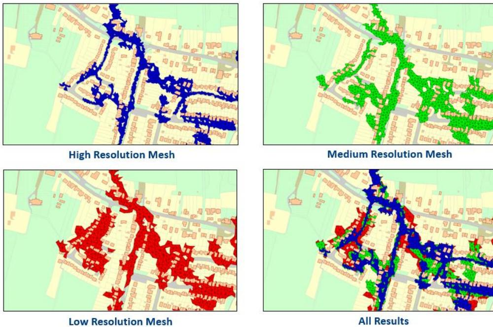
*Figure 2: shows a comparison of the modelled overland flows and the impact on predicted risk when different resolutions of mesh parameters are used.*
