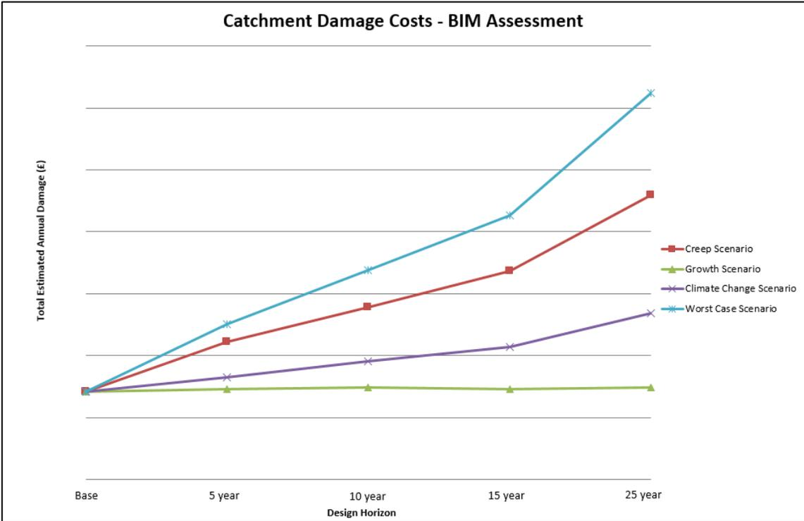
Figure 4 shows the predicted worsening in Total Estimated Annual Damage for an example catchment for each scenario and Design Horizon assessed.
