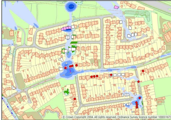
Figure 7: Example of predicted risk of sewer flooding. Red dots indicate properties that have experienced flooding on the HFRR and the blue areas are the extent and depths of predicted flooding from sewer.
