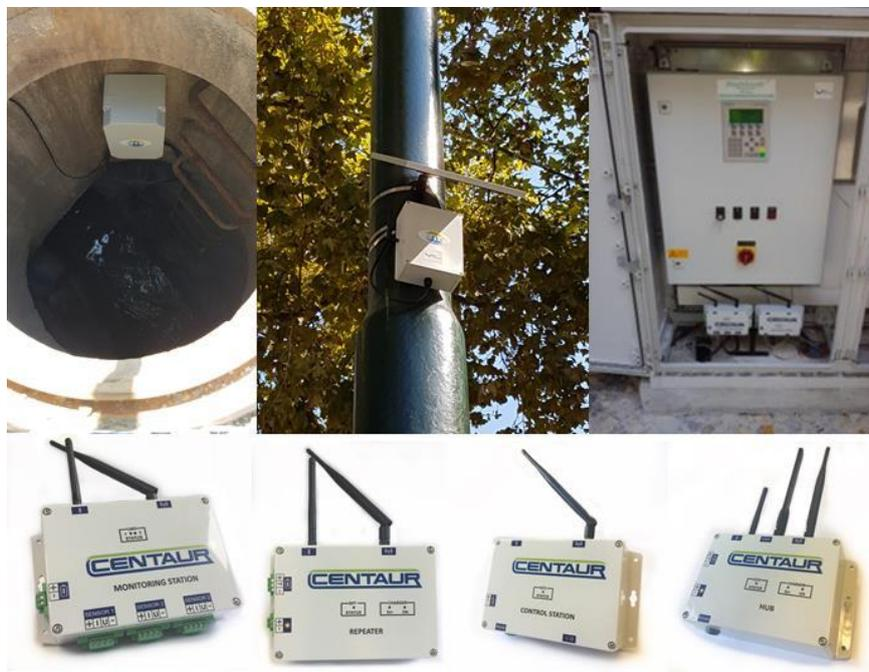
Figure 1: Modular Arrangement of CENTAUR (beta version)
