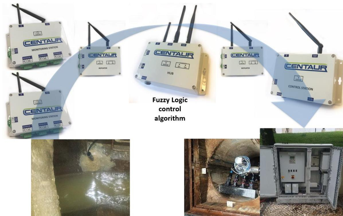
**Figure 1: Modular Arrangement of CENTAUR (beta version)**
