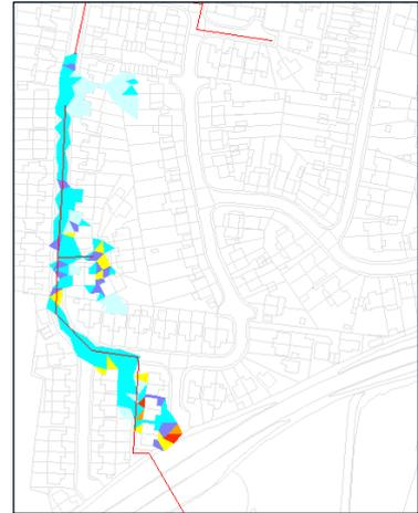
As the scheme increased in size due to the change to the circular liner method, the option was constantly challenged for budgetary reasons. The modelling approach was therefore changed to 2D, modelling a simple mesh over the model to quantify the overland flow paths. This was used to compare the baseline against the proposed option and to help determine and understand the above ground risk and whether the option was definitely needed.
