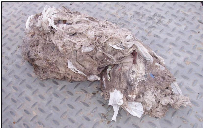
*A sewer blockage removed intact. This shows that wipes were main component*
